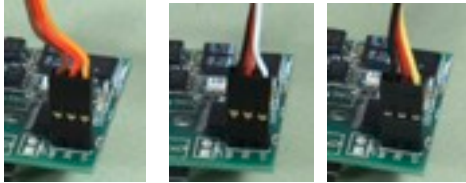
The 3 most common servo lead colors and how they plug in.
