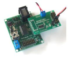
The Octocoder allows you to add eight DCC addresses to the Octopus so that you can throw turnouts/ accessories. Connections are provided for local controls so you can have both DCC and local control at the same time. The stationary decoder is about as simple as they come - there are no CVs to program, just attach and set the address with the address jumper.
