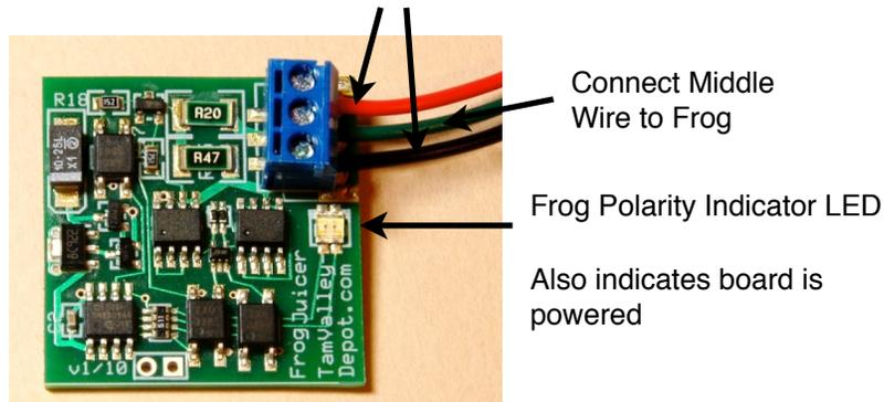
Use #22 - #26 ga. wire and keep the runs under 3 feet. The Frog Polarity Indicator LED will change color when a train crosses a frog that needs to be switched. There should be no interruption of sound or movement when this occurs (unless the track is dirty - sorry - the MFJ can't automatically fix this problem).
