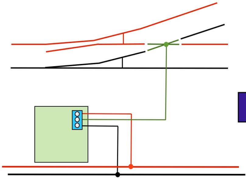
DCC Bus (Direct to command station with no Circuit Breaker between)
